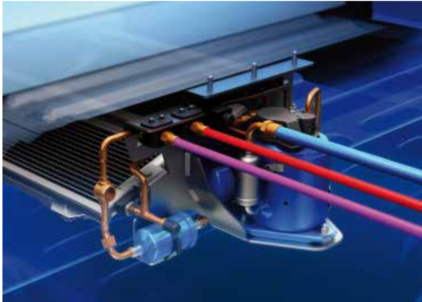
Condenser and compressor built in under chassis
