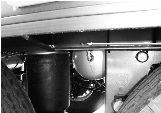
Drain ring (semitrailer left side rail)
