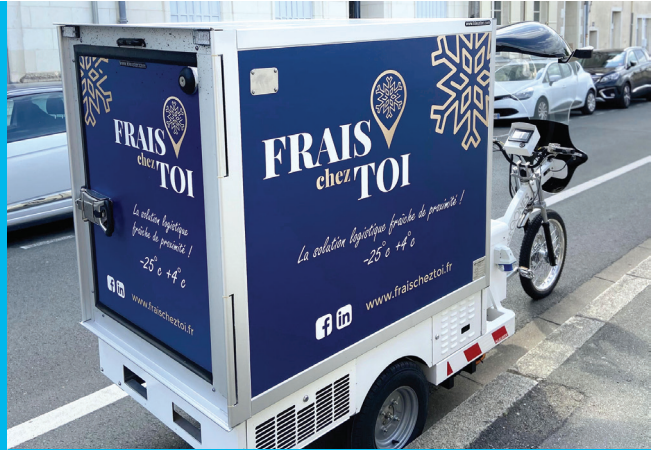
KLEUSTER Freegone is fitted with the new Frigoline body cell with coefficient K 0.31 and positive cold plug & play cooling unit.
