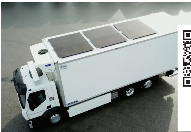
Lamberet has fitted the body roof with 6 solar panels giving a surface area of 10 m 2 providing peak power of 2400 W.
