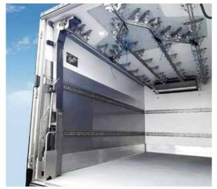
Distributing meat in sides requires specialized assisted unloading tools in order for the driver to handle the job safely. BEEFLIFT is a genuine "Cobot" that replaces the ladder technique: this controlled hydraulic arm provides effortless unloading of 250 to 500 kg carcasses. Developed and manufactured internally by Lamberet, it is 100% stainless steel in order to meet health and hygiene regulations.
