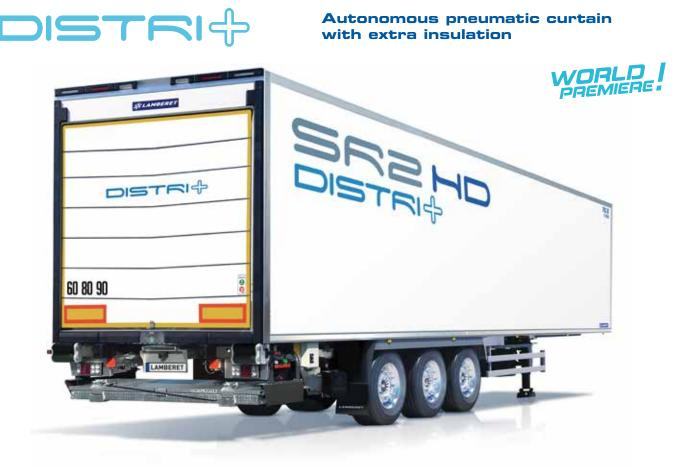
The new Distri+ pneumatic roller shutter door, 100% made by Lamberet, opens up new horizons in distribution. It combines the best useful height/overall height ratio, the widest passageway on the market with 2.42m thanks to its recessed sliders, and the first insulated bed developed for sub-zero applications.
