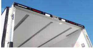
Optimised aerodynamics with a smooth rear, and front Cx Profiles
