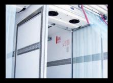
Partitions: these allow several compartments to be created and both fresh and frozen foodstuffs to be transported. They can be fixed lengthwise or crosswise with or without a door, or else sliding crosswise and lifting with the aid of gas struts.
