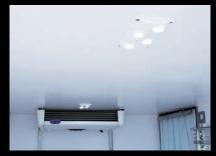
**LED lighting**: An LED overhead light (two if the interior measures over 3.90 m) guarantees exceptional illumination, low electricity consumption and great durability. It is extra flat, just like the switch plate, thus preventing it catching on packages or handling appliances.
