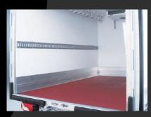
New Frigoline Beef: (illustration: New Frigoline Pro Beef) specially designed for transporting meat, this version is fitted with a reinforced roof for attaching a hanging device appropriate to your activity: a bar with hooks, a sliding hanger, two-rail hanger or tube cupboard, with or without connecting section.
