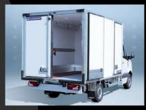
2 (TO2) or 3 (TO3) Leaf Total Back Opening: take advantage of the integral headroom to facilitate loading of panels for posts.
