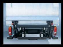
Tailgate elevator: the back of the chassis can be fitted with different forms of tailgate to facilitate your manœuvres: folding tailgates or half-tailgates are available in several loads and dimensions.
