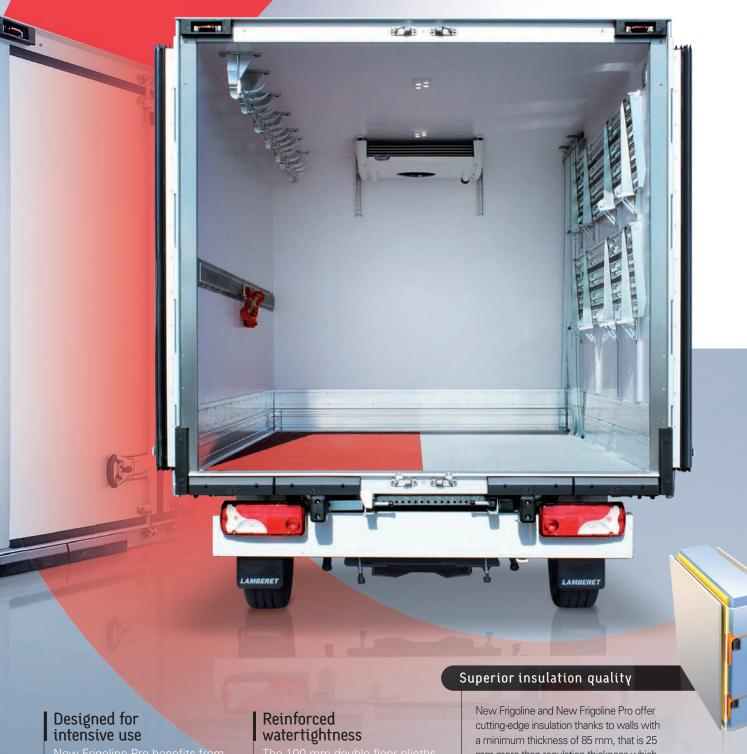
New Frigoline Pro benefits from a reinforced floor made up of two crossed backing plates 6.5 mm thick, designed to bear the heaviest loads. The frame is protected from impacts when handling goods by stainless steel angle bars covering the whole length of the posts.
