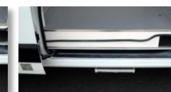
Retractable Quickstep side step (Photo on RWD)
