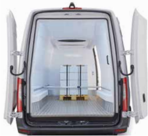
Space between wheelbase compatible with Europalette dimension (single wheel)
