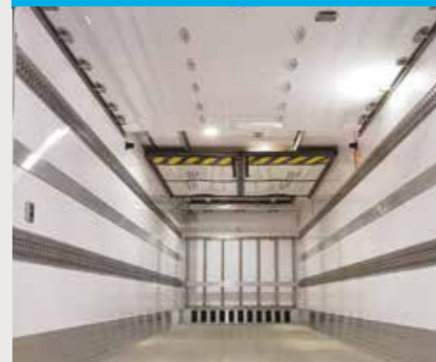
The Distri+ roller shutter door with pneumatic assistance offers entirely automated locking and unlocking: no need to bother with a handle anymore!
