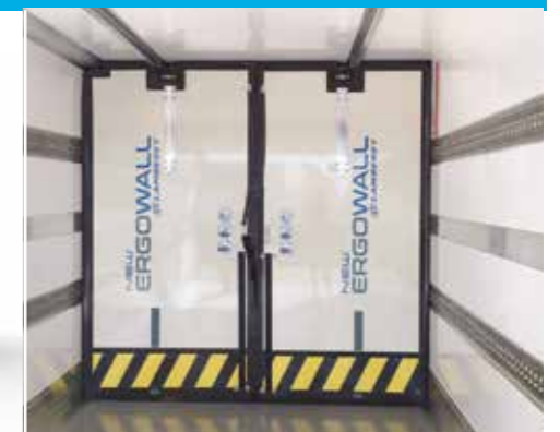
Ergowall, winner of the Trailer Innovation Award: ultra-light bulkheads with enhanced sliding and lifting assistance.
