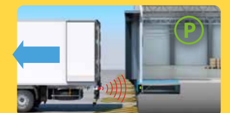
6. Dock ramp folded, TAG hidden, brake vehicle released. Authorized departure.
