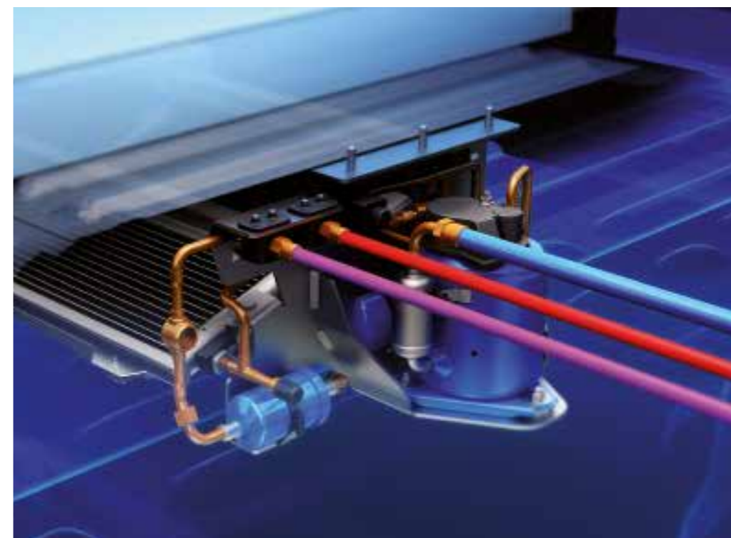
Condenser and compressor built in under chassis
