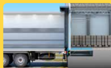
2. Dock ramp unarmed, no signal picked up by RFID radar, unlocked vehicle brakes
