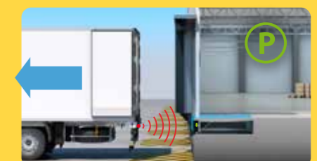
6. Dock ramp folded, TAG hidden, brake vehicle released. Authorized departure.
