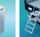
The retractable Safestair step secures the entry and exit of refrigerated trucks and semi-trailers.
