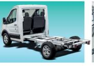
Highly valued for urban distribution and catering, the 3.5-ton platform cab offering is expanding with the launch of the Frigoline body on the Ford Transit modular chassis. This solution features a low floor and a higher payload capacity than traditional chassis cabs.
