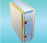
Lamberet is gradually deploying a higher level of insulation in its bodyworks with the new HPI foam, free of HFOs, offering enhanced thermal performance thanks to an 11% reduction in the lambda coefficient
