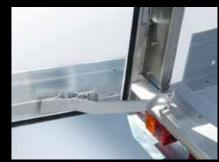
Lamberet trailers have a door retainer (made of rubber or T-shaped, depending on the model
