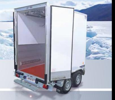
Offering 5 to 7 m<sup>3</sup> of useful volume, this is a true customizable vehicle based on your activity and suited to the transport of large-volume perishable foodstuffs. In its "meat door" version with full rear opening, meat hooks, extra useful height, and red-tinted no-slip floor, this is the ideal solution for meat industry professionals.
