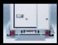
Built into the 750 kg version or a Built into the 750 kg version or attached onto the 1300 or 2000 kg version, the fixed steel "one-level" no-slip foot-step makes it easier
