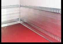
Securing rails and runners (optional): The aluminum runners protect the walls from repeat impacts. The securing rails secure and stabilize your goods during transport (available for round aero type perforations or mixed).
