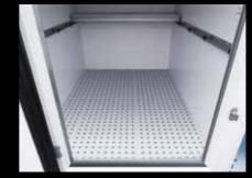
Grating (optional): The floor is covered with removable, slatted plastic slabs, which are easy to wash, in order to allow optimized ven-tilation, prevent contact between food items and the argument and parter the organ food and the ground, and protect the cargo from
