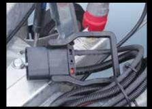
hal), the electrical unit is conn means of a "fenwick" plug to the pulling cle's battery, whose alternator must h
